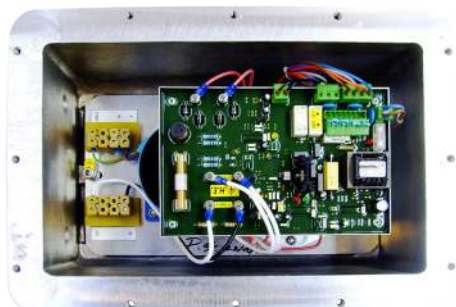
Heavy Duty power unit in certified ATEX enclosures
