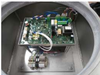
Heavy Duty power unit in certified ATEX enclosures
